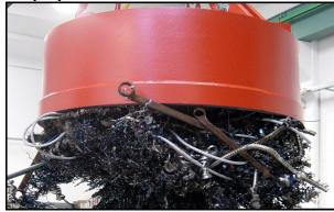
Part # 10-0011 ESB 36 Voltage 24 Volts 80 Amps **Amps** Drop Time 2 to 5 sec - adjustable Weight 1874 Lbs Lift Capacity - loose 600 to 750Lbs Lift Capacity - solid 8,000 plus Lbs *75%* Duty Cycle
