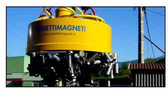
$ESB 32 \qquad Part \# 10-0010$   $Voltage \qquad 24 \ Volts$   $Amps \qquad 40 \ or \ 80 \ Amps$   $Drop \ Time \qquad 2 \ to \ 5 \ sec \ - \ adjustable$   $Weight \qquad 1058 \ Lbs$
